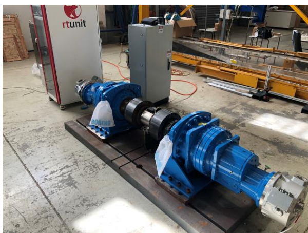
Fig 6. PTO assembled for dry testing.
