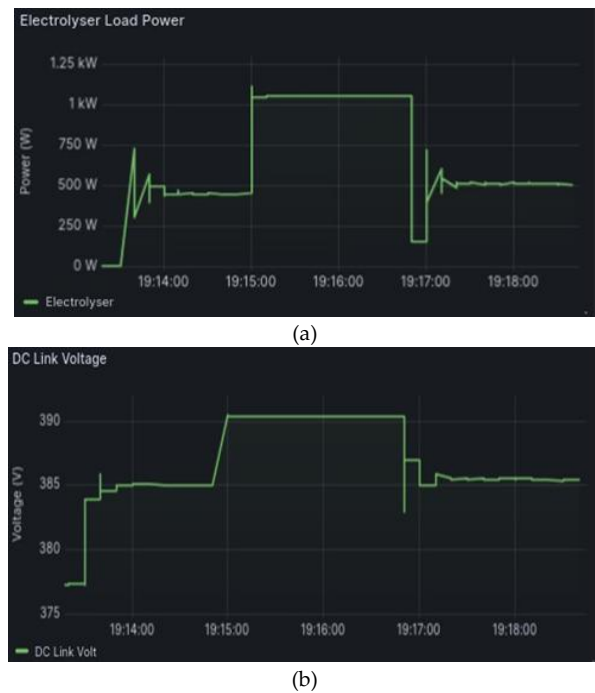
Fig. 7: Operation of (a) Electrolyser and (b) DC link voltage
