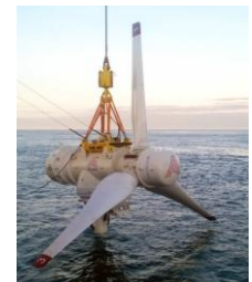
Figure 2: SIMEC Atlantis 1.5MW Tidal turbine [5]
