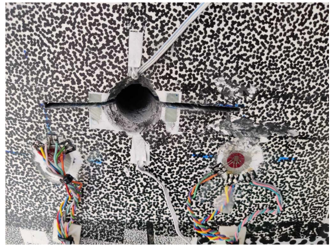
Fig. 5. Installation of Strain gauges around hole and notches in the blade.
