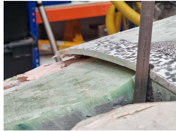
Fig. 12. Thick adhesive layers (green) averaging 10 mm thickness, showing debonding from the GFRP blade skin.
