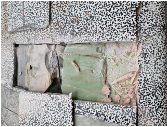
Fig. 14. Image showing a section of blade with the outer skin removed. From bottom to top: leading edge of blade, pink coloured filler at overlap seam, green Spabond adhesive, black carbon spar.
