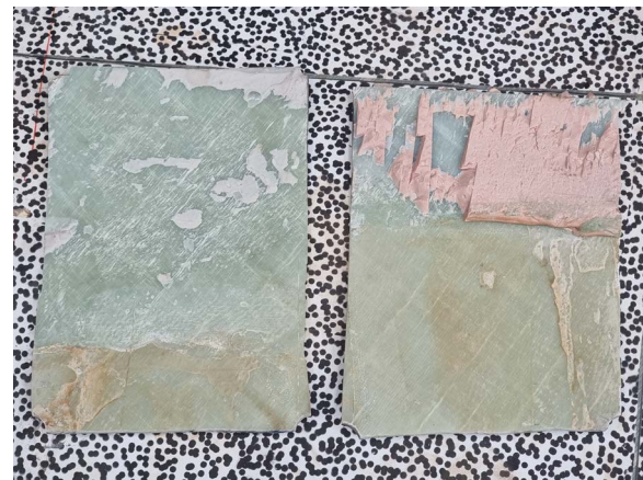
Fig. 13. Cut away blade skin showing inadequate bonding between the blade skin and core structure.
