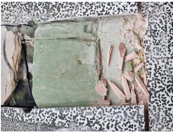
Fig. 15. Section through blade skin showing voids in between adhesive bond lines. Adhesive thickness at this location is approximately 15 mm.
