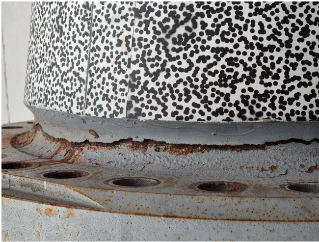
Fig. 6. Image of failed blade root showing crack from delamination extending around the circumference of root connection.
