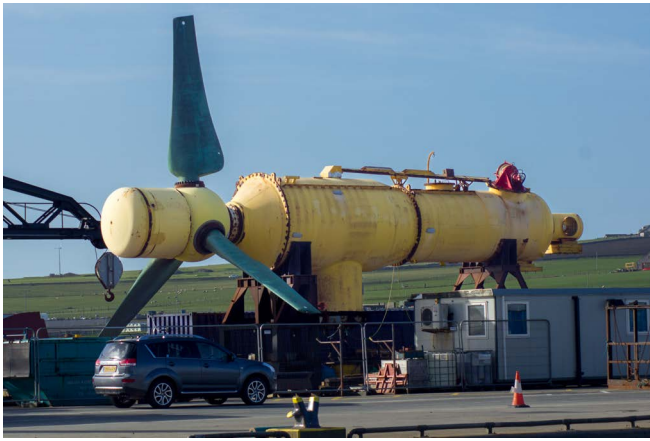
Fig. 1. DeepGen III Tidal turbine after being removed from the Fall of Warness site, showing the tidal blades, one of which was tested at FastBlade [9].
