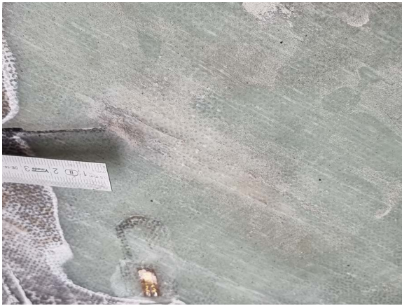
Fig. 11. Visible cracking in composite surface running at 45° from the tip of the notch. Ruler and notch at image right orientated in chordwise direction.
