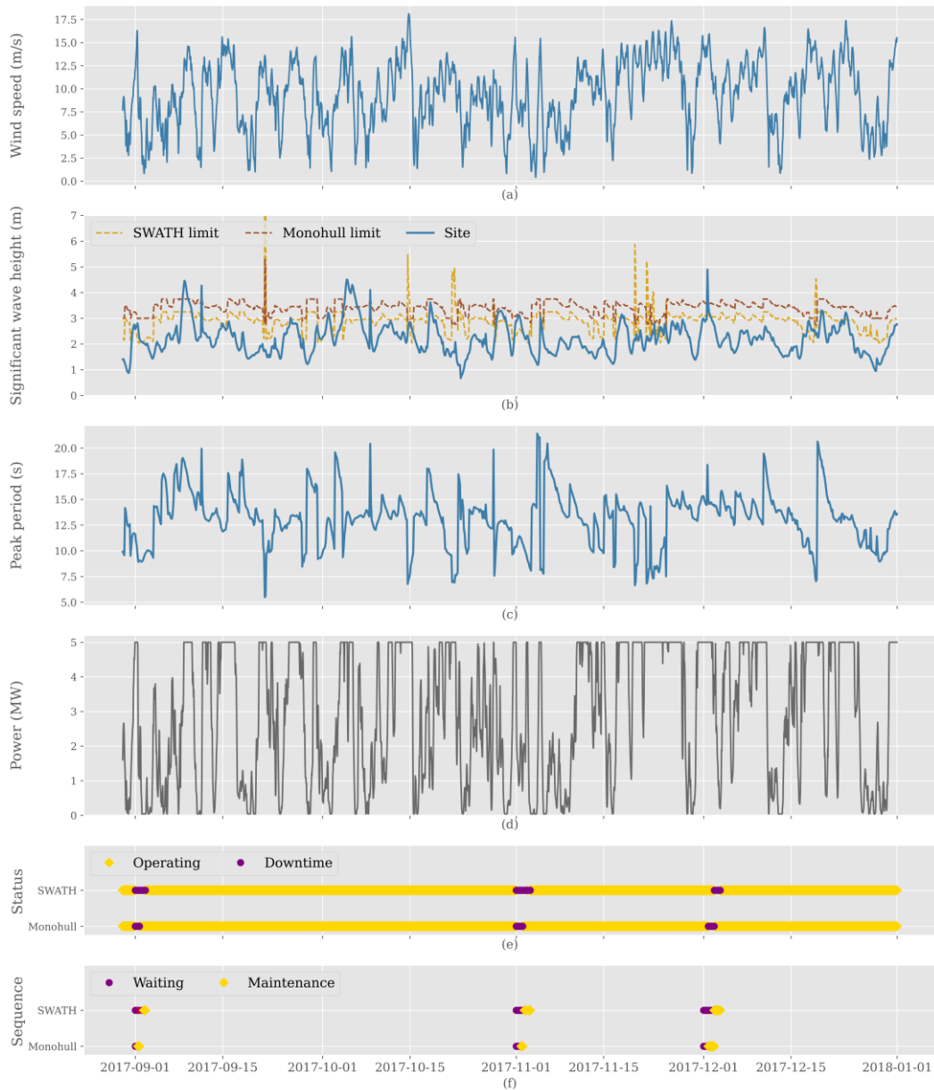
Fig. 6. Visualisation example of discrete event simulations results, for a selected period (Sept. to Dec. 2017).
