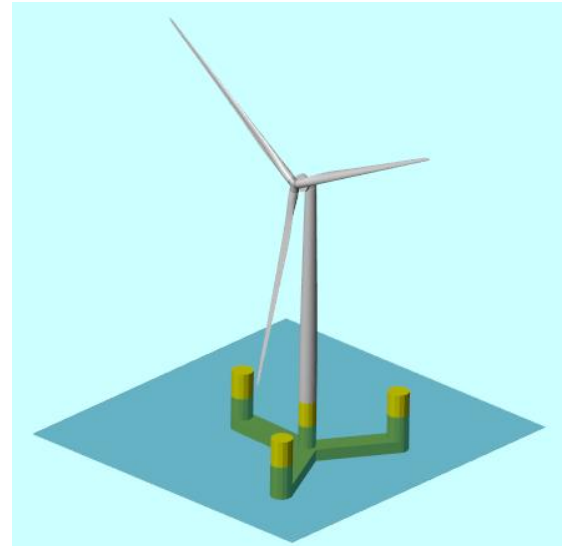
Fig. 5. WEC-Sim+ MOST (Matlab for Offshore Simulation Tool) model of a FOWT used to demonstrate the new QTF feature.
