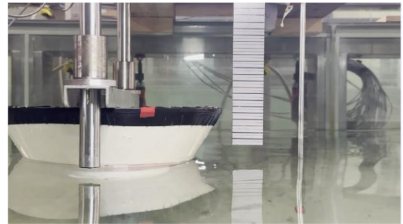
Figure 7 Example of footage captured for free decay and incident wave tests
