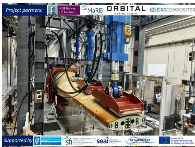
Fig. 2 A large tidal blade installed at the Large Structures Testing Laboratory undergoing structural testing using the multi actuator load introduction system.
