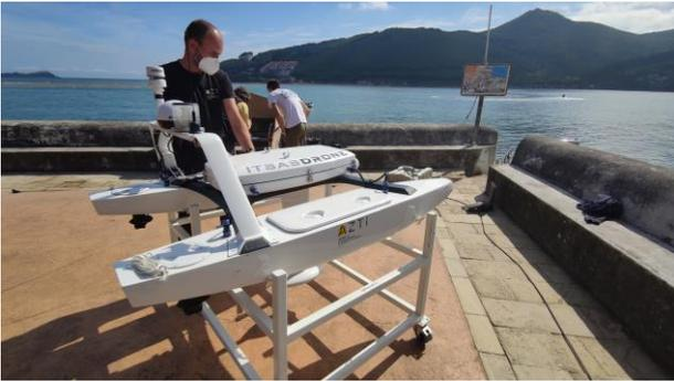
Fig. 1. ITSASDRONE, an autonomous marine surface drone (Source: AZTI).
