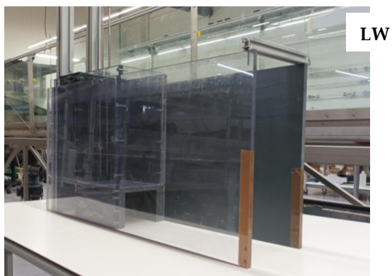
Fig. 7. Lateral wall (LW) with heights of 364 mm installed in the Mutriku power plant.
