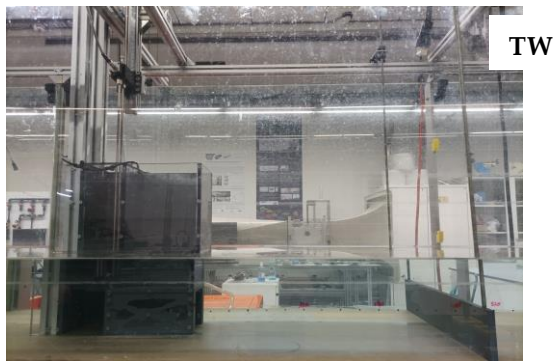
Fig. 6. Transversal wall (TW) of 80 mm installed in front of the model representing the Mutriku power plant.
