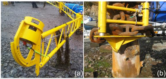
Fig. 5. Panel (a): ADP protective mounting bracket with manually adjustable pitch angle. Panel (b): C-ADP frame foot.
