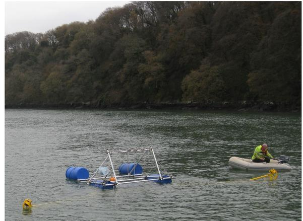
Fig. 3. Deployment raft and C-ADP onsite at Warrior Way prior to seabed deployment
