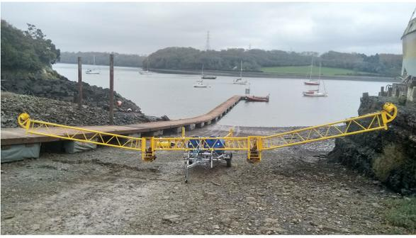
Fig. 1. Fully assembled frame on launch trailer, prior to buoyancy system test. ADP mounting points are shown at end of arms, but sensors are not installed in this image.
