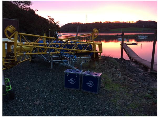
Fig. 2. Frame with arms folded for storage and movement
